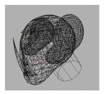
Modelling: Chin, Head and Ears are made of Meta Balls. The Mouth is cut into the face by a cookie
