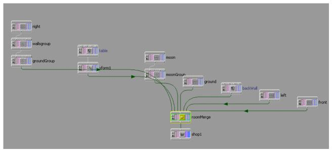
Modelling: The window of the room is made by a *Cookie Operation* by which the window is cut out of the back wall (*A minus B*).
